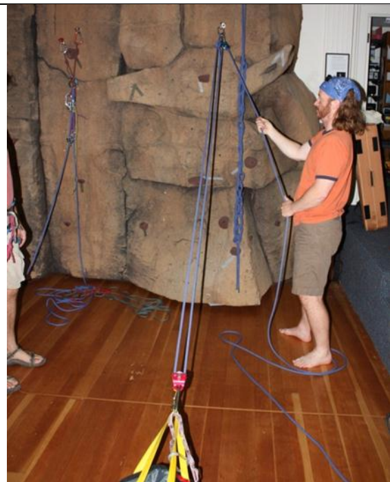
Figure 3.2: A simple 2:1 with a redirect. Note that adding a fixed pulley to the hauling end adds no mechanical advantage, so you don't count that pulley, or the resulting redirect strand.
