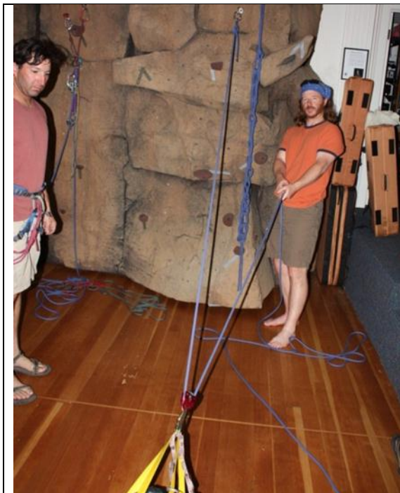
Figure 3.1: A simple 2:1. Note the hauling strand is fixed to the anchor. Count the pulleys (1) and add 1 = 2:1. Count the strands under load (2) = 2:1.
