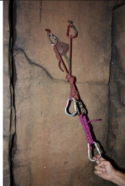
Figure 2.2: Extending the power point
