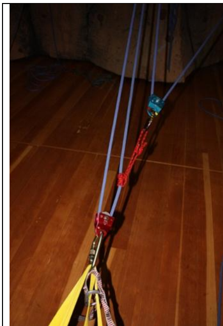
Figure 3.5: This is a detail of the same MAS shown in Figures 3.3 & 3.4. The third pulley has been moved from the load to a prusik chord on the second strand of the original 2:1 MAS. Pulleys no longer move to the anchor at the same rate
