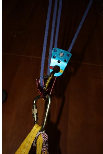
Figure 3.4: 4:1 travelling pulley detail. Both are attached to the load and travel towards the anchor at the same rate (the hallmark of a Simple MAS).
