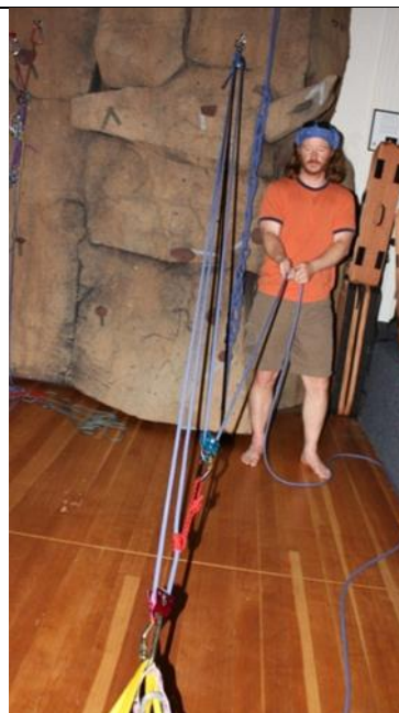
Figure 3.6: Full view of the anchor detailed in Figure 3.5. The strand above the prusik goes to a pulley at the anchor, down to a pulley at the prusik, and back to the hauler, making a 3:1 on a 2:1. This is a 6:1.
