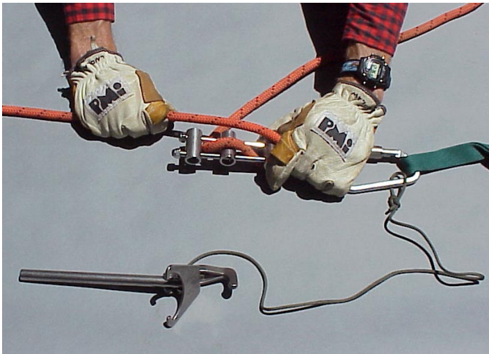
Figure 10 – Nano-Belay and Unloader.
