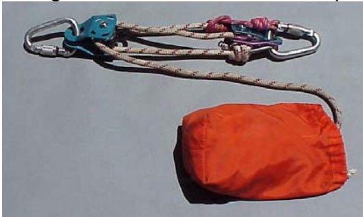
Figure 18 – Attendant Jigger in 3:1 mode with a change of direction.
