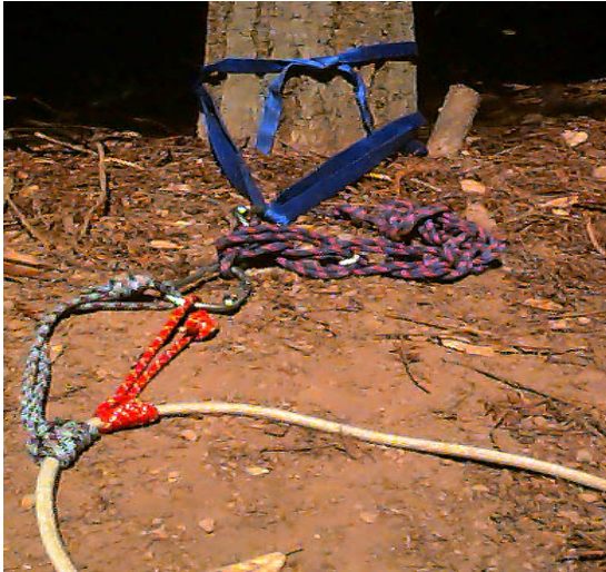
Figure 2 – Wrap Three, Pull Two Anchor
