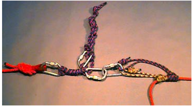
Figure 5 – Tandem Prusik belay attachment, before rigging to belay line and attached to the belay line ( picture incorrect with too many carabiners )
