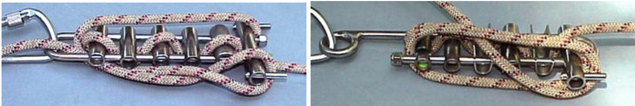
Figure 4 –. Break bar racks, tied off.
