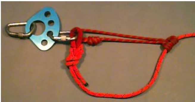
Figure 15 – Using a soft interface at the anchor.
