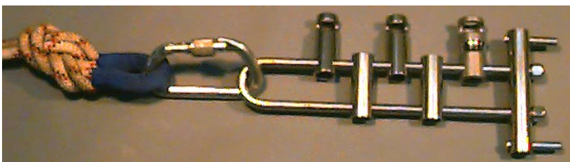
Figure 2 – Break bar rack, before rigging.
