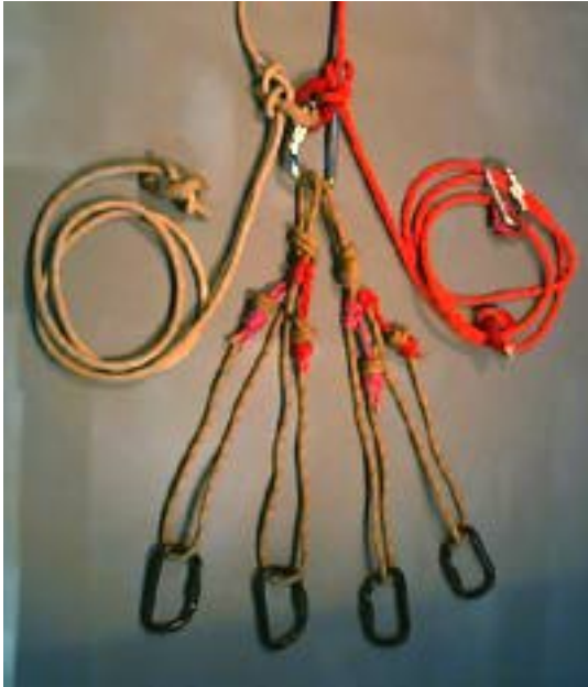
Figure 20 – Homebuilt Spider attachment.
