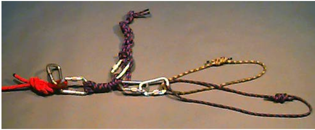
Figure 5 – Tandem Prusik belay attachment, before rigging to belay line and attached to the belay line ( picture incorrect with too many carabiners )
